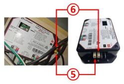
If the reset does not have the desired result, first disconnect the white cable (5) (power connection) from the module and wait for 30 seconds before
